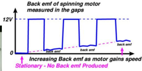
Following on from the <sup>1</sup>/<sub>2</sub>-wave mode of *pre-electronic-era* controllers, early units used the same mains-based 50/60-100/120Hz low frequency for their pulse rate. These are NOT suitable for use with decoder-fitted locos, or 'Coreless Motors' because of the heavy jogging and Buzz effect of the low pulses. A decoder would have to shutdown and then reset on each 100Hz cycle of the waveform.
