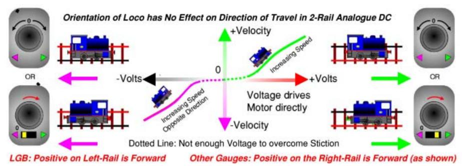
In the 'Traditional'/ Historical Method of DC Analogue Control shown above, a variable d.c. voltage is applied to the track.
