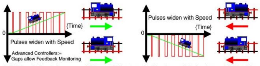
Full Voltage Pulses help overcome Stiction and drive Controller Transistors efficiently. Average V drives Motor
